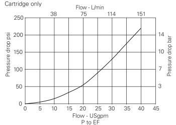
Notes: Minimum inlet flow should not be less than 1/4 of maximum inlet flow. Minimum pressure drop is determined by control pressure.
