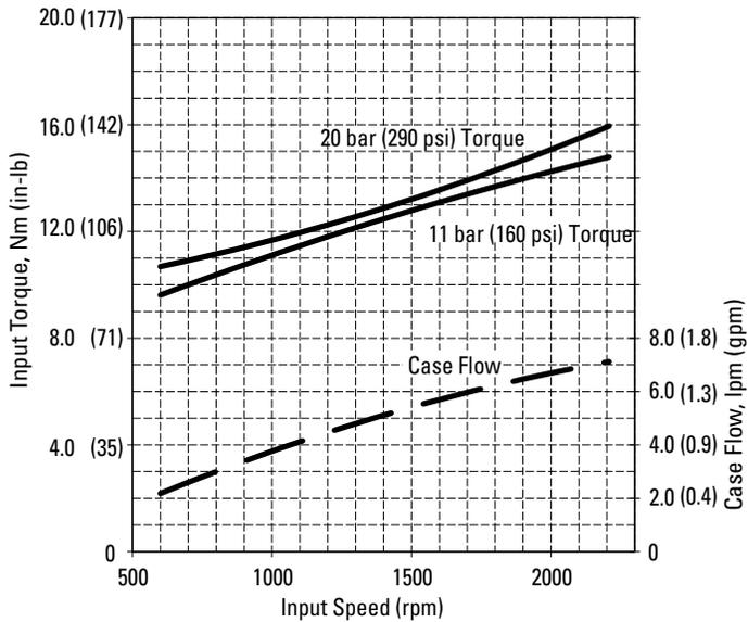
**Input Torque and Case Flow Cut-off @ 49°C (120°F)**
