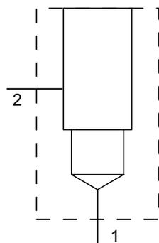
Compatible with the DFB\* family of FLEx valves, Sun Hydraulics offers 31 standard line-mount manifolds in 90°, in-line, through port 1 with gauge port, cross port and direct mount (banjo bolt) versions for the T-162A cavity. Standard products include one- and two-cavity versions in a wide range of port sizes. The popular AAJ model line-mount 90° manifold (shown at left) has a single cavity and SAE 8 ports.
