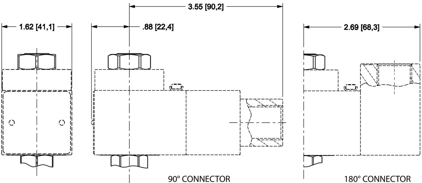
NOTE: Please verify cartridge clearance requirements when choosing a Sun manifold. Different valve controls and coils require different clearances. An additional minimum 2.0 in. (50,8 mm) beyond the valve extension is needed for coil installation and removal.
