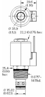
Torque cartridge in steel housing 68-75 Nm (50-55 ft lbs)
