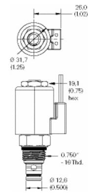
Torque cartridge in aluminum or steel housing 34-41 Nm (25-30 ft lbs)
