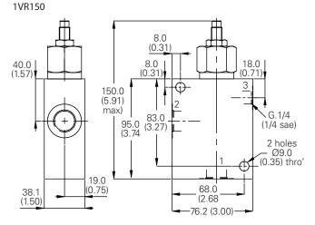
Note: For applications above 210 bar, please consult our technical department or use the steel body option. Note: Tightening torque of "F" adjuster locknut - 20 to 25 Nm
