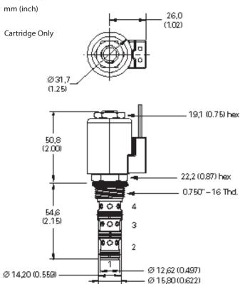
Torque cartridge in steel housing 34-41 Nm (25-30 ft lbs) Note: When solenoid valve is ordered as cartridge only, nut is included.
