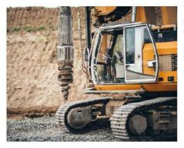
Applications such as mowers, cutters, shears, and augers for example, reap the benefits of this valve. Typically used for drilling methods, the auger screws into soil and material is driven up the shaft of the rotation mechanism.
